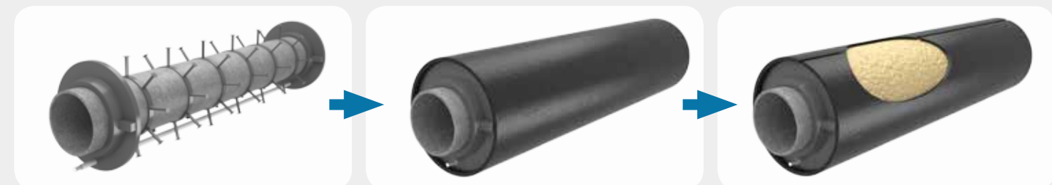
Hostpipe section with spacers, fiber optic cable and endseals installed. Ready for jacket.
