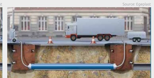
Close-fitting/fixing the liner inside the host pipe using hot steam.
