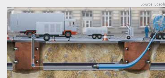
Installation of the factory folded liner inside the host pipe.
